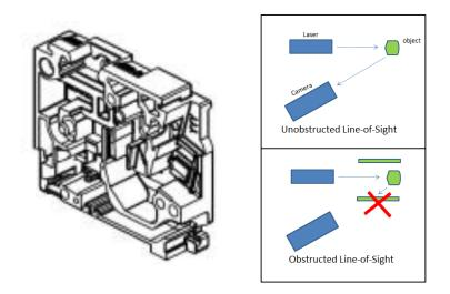
FIGURE 2: Left – an injection molded plastic part with high feature density. Right Top – Typical line-of-sight between the laser, the object being scanned and the camera. Right Bottom – An illustration of an obstructed line-of-sight.
